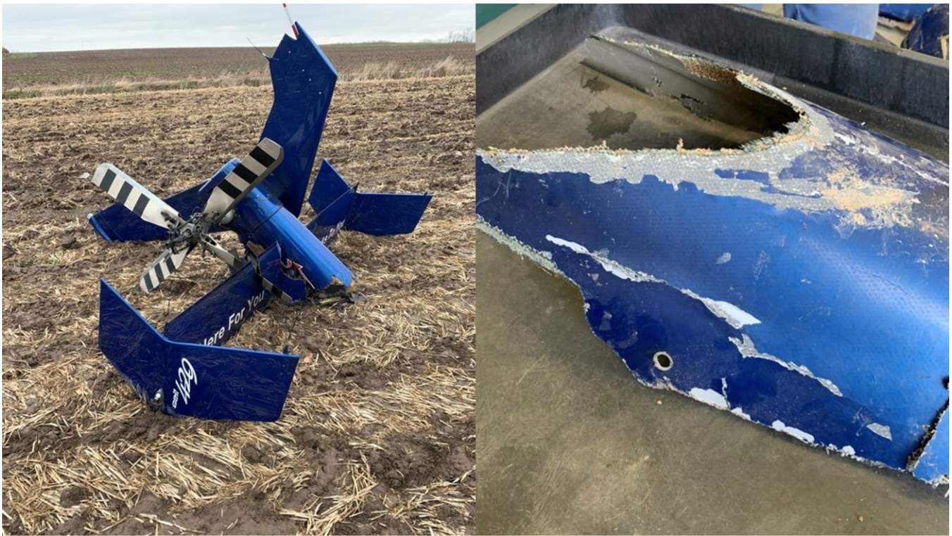
Figure 1 Figure 1 Tail rotor and main rotor blade slice in tail boom.
